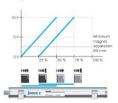
Programming example: Differential travel 50 % nominal stroke = 10 V differential signal
